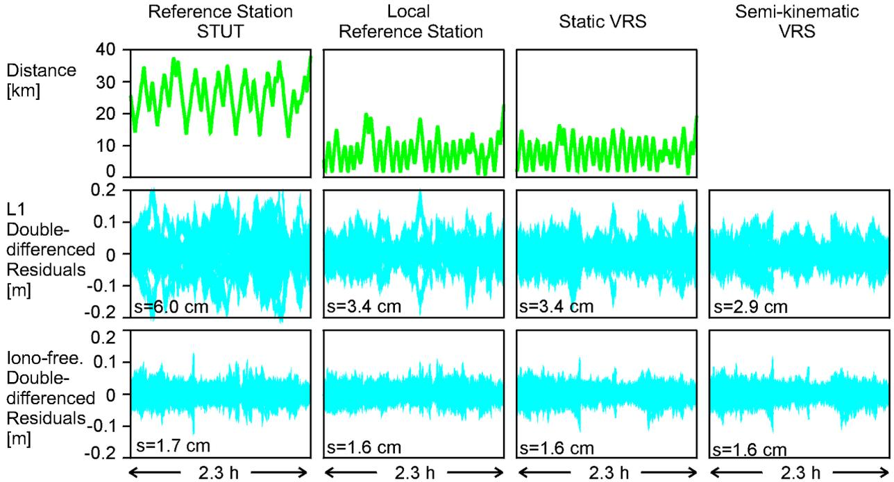
**Fig. 8:** Four different baseline solutions for the observations of test data set 2: distances to the reference stations, double-differenced residuals in the baselines from the reference stations to the rover.
