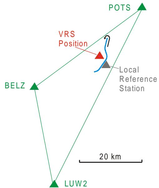
**Fig. 3:** Rovers trajectory and reference stations of test data set 1.
