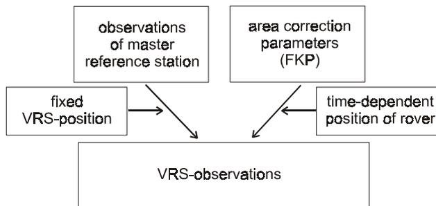
**Fig. 2:** Computation of the observations of a semi-kinematic VRS.
