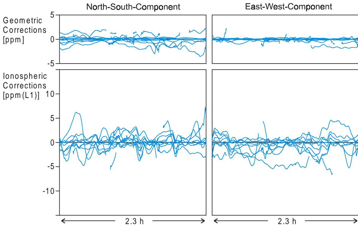
**Fig. 7:** Parameters of non-dispersive (geometric) and dispersive (ionospheric) correction models for test data set 2.
