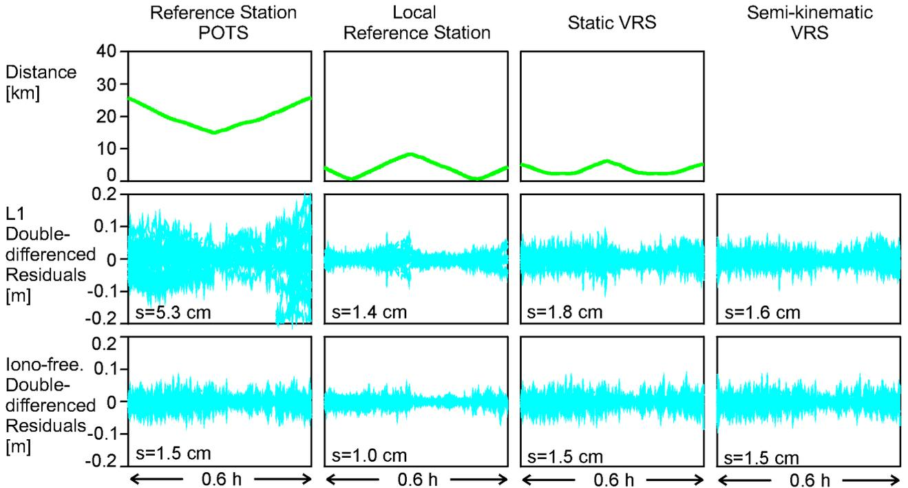
**Fig. 5:** Four different baseline solutions for the observations of test data set 1: distances to the reference stations, double-differenced residuals in the baselines from the reference stations to the rover.
