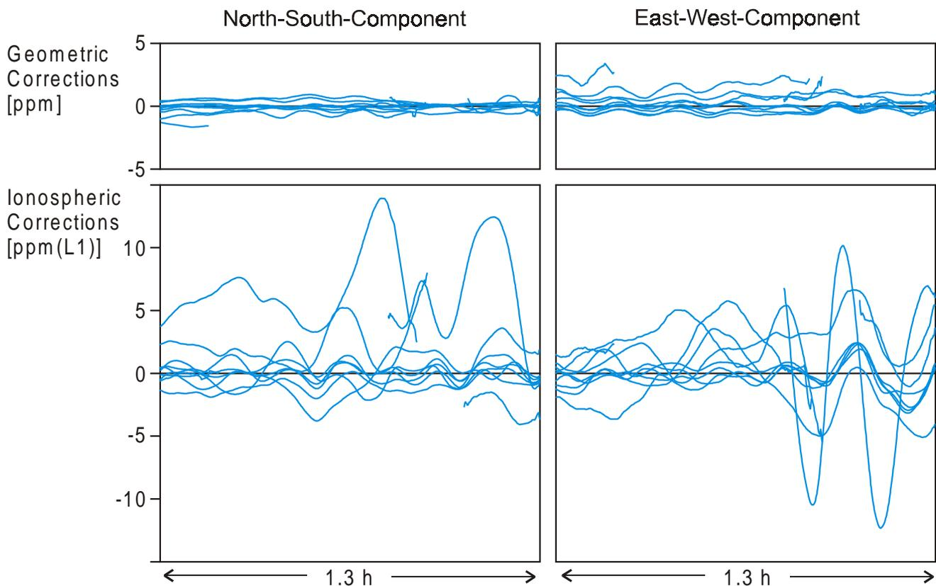
**Fig. 4:** Parameters of non-dispersive (geometric) and dispersive (ionospheric) correction models for test data set 1.
