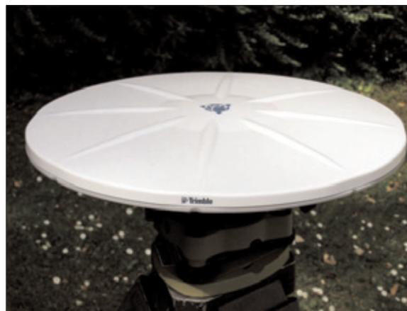
Abb. 9: Trimble-Zephyr-Geodetic-Antennen (TRM41249.00 NONE) (Foto: Galitzki)
