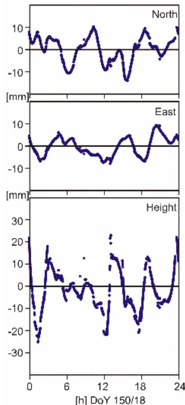
**Figure 7.** Epoch-by-epoch coordinate errors of station BIK0 (Bishkek, Kyrgyzstan) on DoY 150/18 due to L2 quarter cycle biases: ionosphere-free linear combination with ambiguities being fixed, estimation of tropospheric zenith delays enabled.
