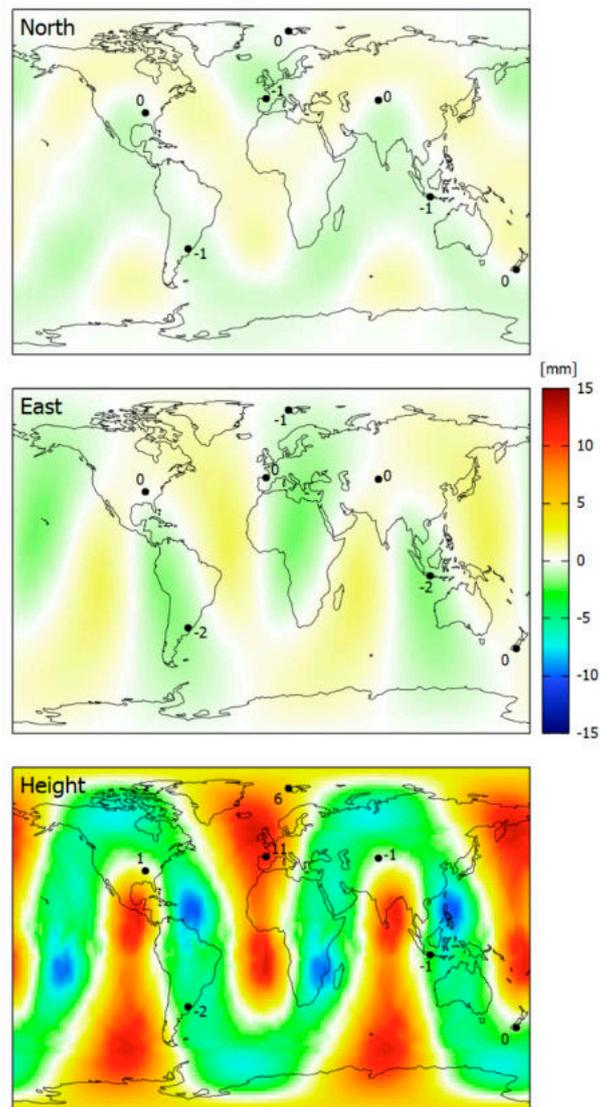
**Figure 6.** Coordinate errors of 24 h static positioning in early 2018 due to L2 quarter cycle biases: ionosphere-free linear combination with ambiguities being fixed, estimation of tropospheric zenith delays enabled, based on simulated stations in a  $2^\circ \times 2^\circ$  grid and on seven real stations.
