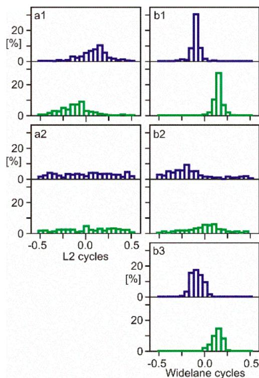
**Figure 2.** Distribution of fractional ambiguities of unaligned L2P(Y)/L2C carrier phase observations: (a1) L2, short baseline, (a2) L2, long baseline, (b1) WL, short baseline, (b2) WL, long baseline, (b3) Melbourne-Wübbena linear combination, PPP; each panel consists of 2 sub-panels: upper sub-panels refer to L2C, lower sub-panels refer to L2P(Y); the bin width is 0.05 cycles.
